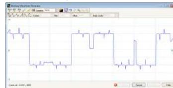
generator. Waveforms can be created or edited using the built-in AWG editor, imported from oscilloscope traces, or loaded from a spreadsheet.
