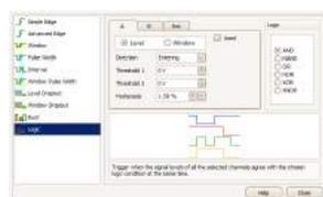
As well as the standard range of triggers found on all oscilloscopes, the PicoScope 5000 Series offers an industry-leading set of advanced triggers including pulse width, windowed and dropout triggers to help you capture the data you need.
