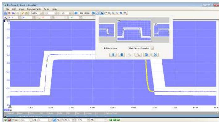
Connect the system under test, and PicoScope will highlight any parts of the waveform that fall outside the mask area. The highlighted details persist on the display, allowing the scope to catch intermittent glitches while you work on something else. The measurements window counts the number of failures, and can display other measurements and statistics at the same time. You can import and export masks as files.
