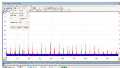
With a click of a button, you can display a spectrum plot of the selected channels with a maximum frequency up to 200 MHz. A full range of settings gives you control
