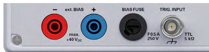
Fig. 4.2: Rear panel with fuse
