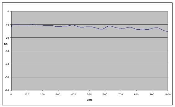
Response of the DUT terminals to the RF output line (outgoing to the DUT) if a constant RF voltage is supplied to the DUT terminals – total frequency range, constant characteristic, drop in the upper frequency range
