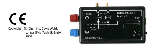
Measurement of conducted disturbance emissions in board networks
