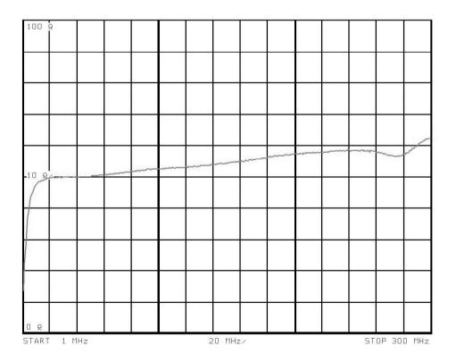
Impedance on the negative measuring line (outgoing to the DUT) if the negative RF measuring channel is terminated by 50  $\Omega$  (ground switch is open)
