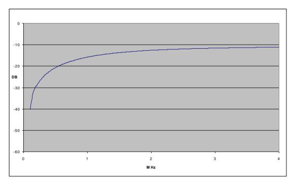
Response of the DUT terminals (outgoing to the DUT) to the RF output line if a constant RF voltage is supplied to the DUT terminals – lower frequency range, rising characteristic
