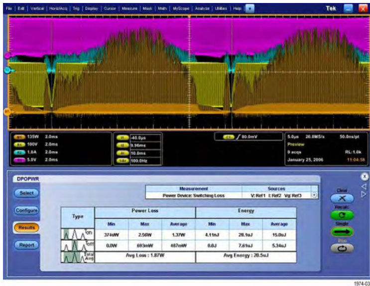
Figure 5: Switching loss results display
