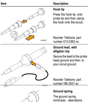
minimizes aberrations on high-frequency signals caused by the inductance of the ground path, giving you measurements with good signal fidelity. Attach the spring to the ground band on the probe
