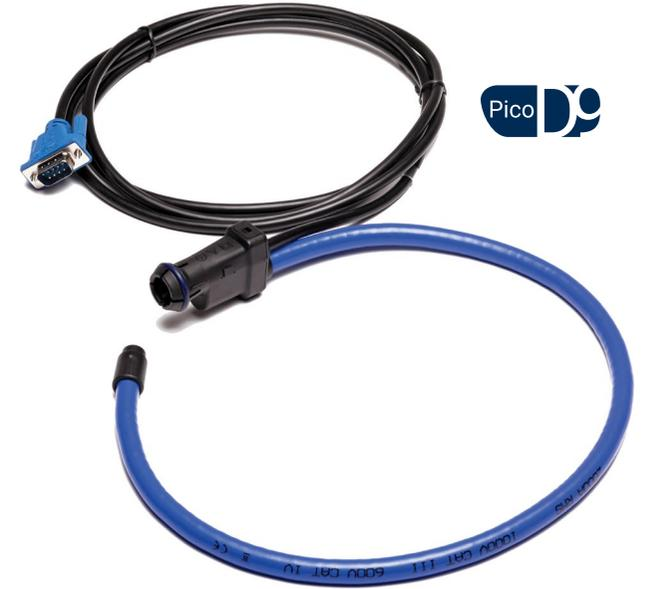
The TA368 is a 2000 A AC RMS probe with 10 Hz to 20 kHz bandwidth, rated to 1000 V CAT III and 600 V CAT IV on uninsulated conductors. It has a flexible sensor coil, enabling you to measure currents on hard-to-reach conductors.
