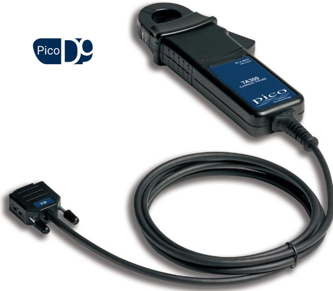
The TA300 current probe is a 40 A AC/DC probe with 100 kHz bandwidth. It is a precision probe for smaller currents, rated for use up to 300 V CAT III on uninsulated conductors.
