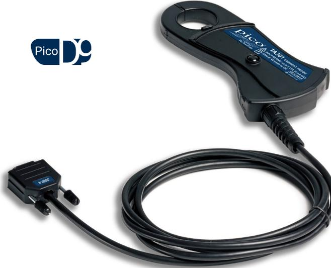
The TA301 current probe is a switched-range 200/2000 A AC/DC probe with 20 kHz bandwidth, rated to 150 V CAT II on uninsulated conductors.
