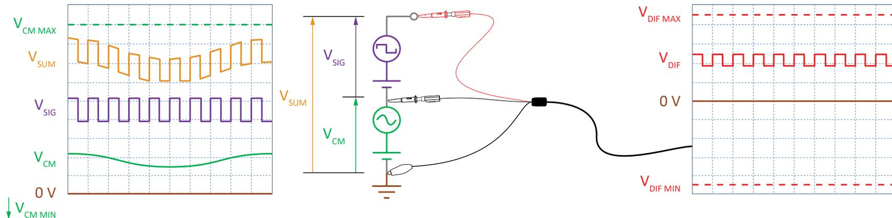
Differential scopes can measure the AC or DC voltage between two points connected to the positive and negative leads, when neither of the points is grounded. This enables them to take measurements where single-ended scopes can't, for example at voltages that are much higher than ground potential. The resulting measurements focus exclusively on the potential difference between the probes.
