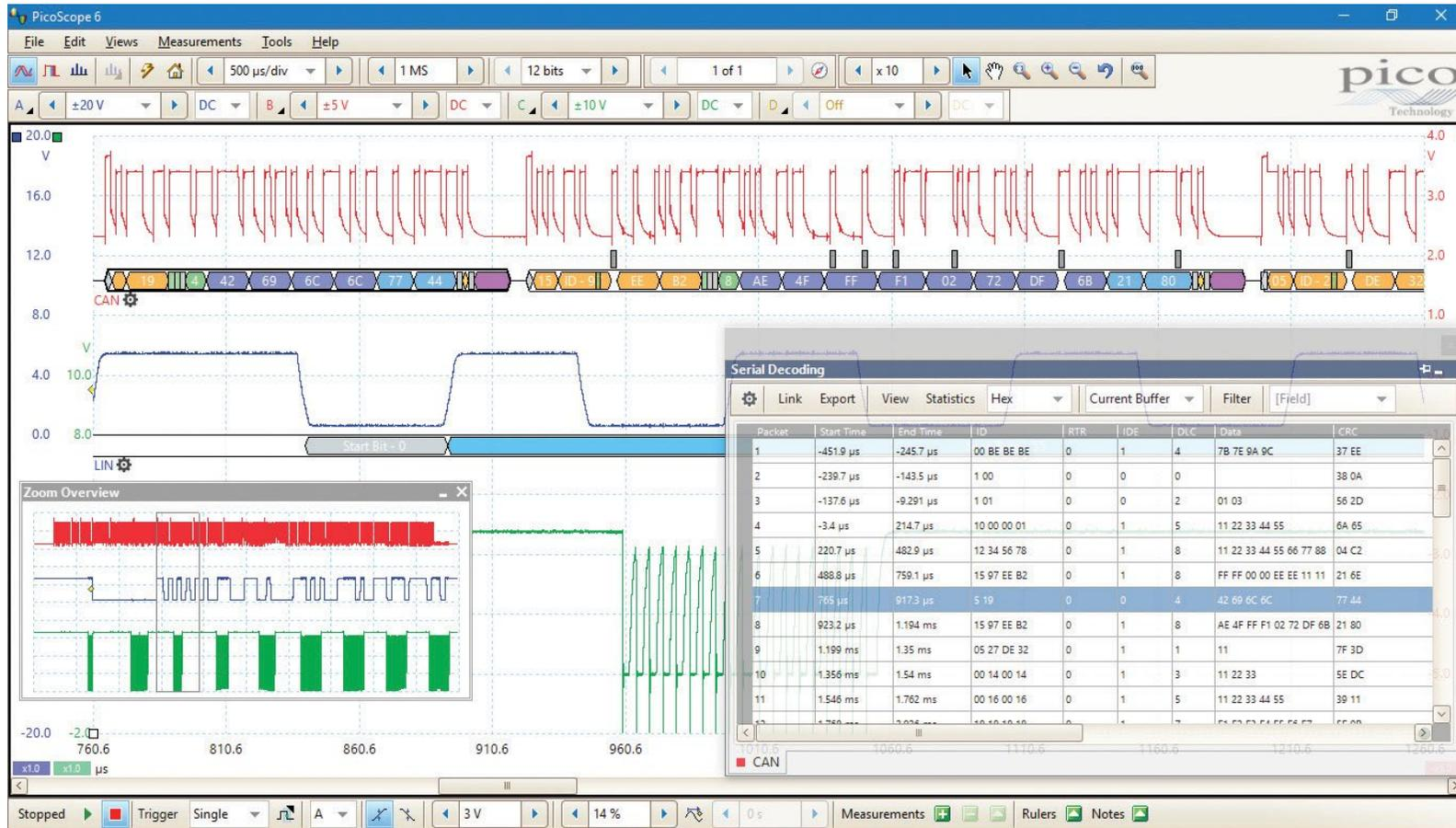
**Graph format** shows the decoded data (in hex, binary, decimal or ASCII) in a timing diagram format, beneath the waveform on a common time axis, with error frames marked in red.
