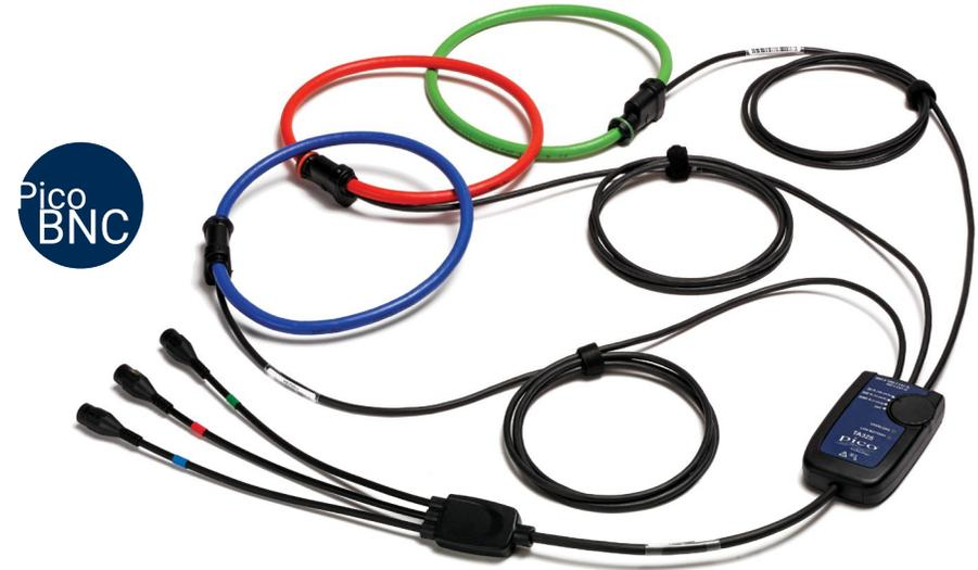
The TA325 is a switched-range 30/300/3000 A AC RMS probe with 10 Hz to 20 kHz bandwidth, rated to 1000 V CAT III on uninsulated conductors. Suitable for measuring 3-phase AC current, it has three sensor coils and scope connection leads, color-coded to match Channels A, B and C in the PicoScope software. Typical battery life is 1000 hours.
