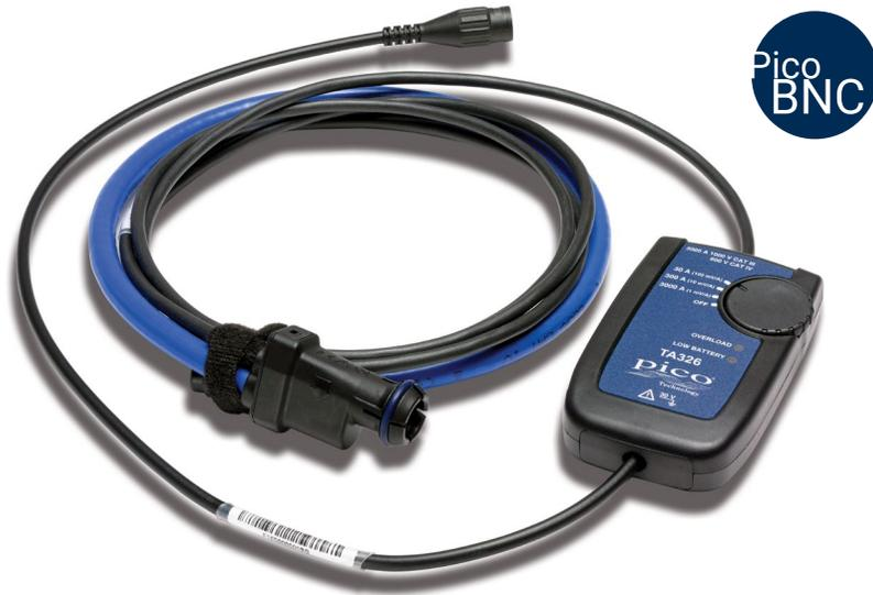
The TA326 is a switched-range 30/300/3000 A AC RMS probe with 10 Hz to 20 kHz bandwidth, rated to 1000 V CAT III on uninsulated conductors. Typical battery life is 2000 hours.
