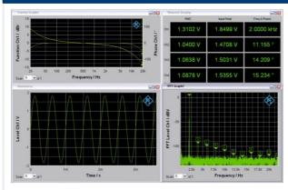
Everything at a glance: Multiple measurement diagrams can be arranged in any desired configuration on the screen; analyses in the frequency and the time domain can be displayed simultaneously.
