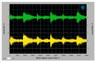
Complex test signals from WAV files can be output at all interfaces; in this example, the waveform function shows the time characteristic of a dualchannel music signal.
