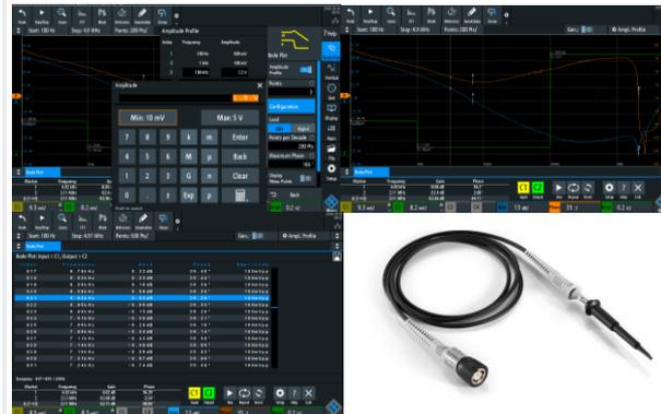
Easily and quickly analyze low frequency response on your oscilloscope with the R&S®RTx-K36 frequency response analysis (Bode plot) option. This option uses the oscilloscope's built-in waveform generator to create stimulus signals ranging in frequency from 10 Hz up to 25 MHz. Measuring the ratio of DUT signal input and output at each test frequency, the oscilloscope plots gain and phase logarithmically.
