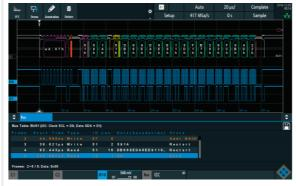
You can analyze the decoded bus frames by overlaying the signal with color-coded data. Address and data content can be displayed in hex, bin or ASCII format. Turning on a bus table makes it easier to see the contents of multiple packets. This can be very useful when zoomed out on the oscilloscope. You can also export the table.
