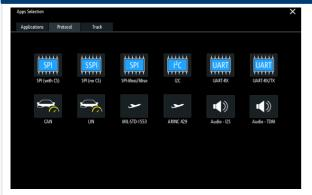
Any protocol can be configured in a few steps from the app cockpit. Once the bus to be decoded and the connected channels have been selected
