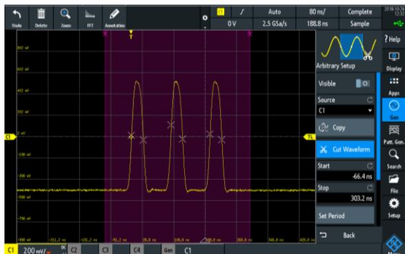
Testing your device with real-world signals opens up a new method to test the margins of your design. The R&S®RTx-B6 arbitrary waveform generator lets you cut waveforms (move the purple lines on the display to set the start and stop) and load them into the arbitrary waveform generator. This allows you to select a portion of a captured oscilloscope waveform in the arbitrary setup.
