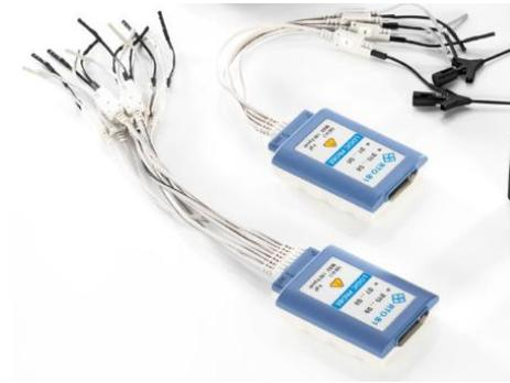
The digital inputs are grouped into logic probes with eight channels. High input impedance combined with low input capacitance of 100 kΩ || 4 pF ensures high signal fidelity and low loading of the test points.
