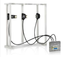
Accurate, secure placement of antennas ensures repeatable measurement results.
