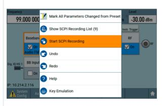
The integrated SCPI macro recorder has a built-in code generator that allows users to automatically record all manual settings and create a directly executable MATLAB® script.
