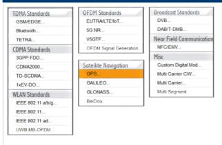
Modulated signals for different standards can be generated with the R&S°WinIQSIM2 $^{TM}$  simulation software. The software supports wireless standards such as 5G and LTE and the generation of noncellular signals such as Wi-Fi (IEEE 802.11xx) and many others.
