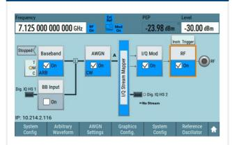
Instantly see the signal flow in the R&S®SMCV100B as well as the status of instrument inputs and outputs. An integrated graphic function displays the generated signal in real time.
