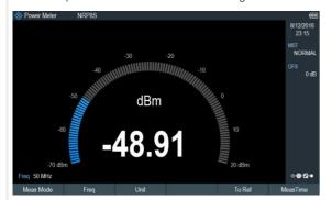
Power measurement with the R&S®NRP8S power sensor
