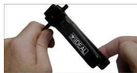
3. Rotate stripper in direction of lettering
