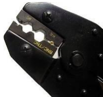
2. Place center contact pin point down into smallest crimp nest
