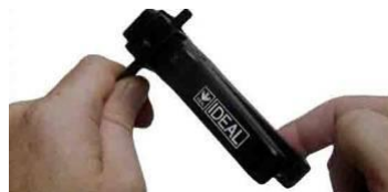
3. Rotate stripper in direction of lettering
