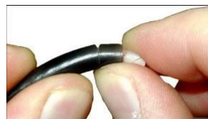
6. Remove 3 rd slug by bending cable
