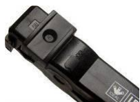
1. Set sliding window to cable size
