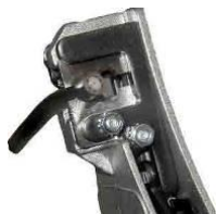
1. Place cable in smaller hole 1/2" protruding
