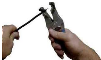
2. Squeeze handles together firmly & quickly
