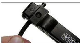
2. Place cable in stripper with 1/4" protruding
