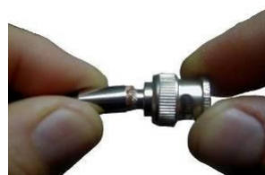
2. Seat the ferrule against the connector body with equal, opposing force
