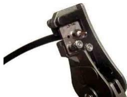
3. Place cable in larger hole 1/4" protruding, squeeze
