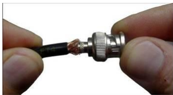
1. Seat connector body onto dielectric, underneath the braiding, listen for click of captive contact pin
