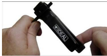
4. Check by restripping cable. What was the left side is now the right side upside down!
