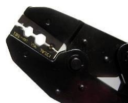
Wrong side up
