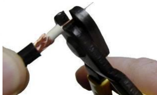
2. Lay side of cutter against white dielectric
