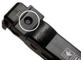
1. Set sliding window to cable size
