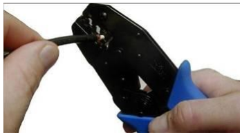
3. Place center conductor all the way into center contact pin and crimp
