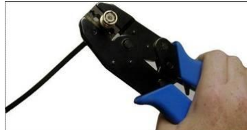
3. Squeeze handles together completely
